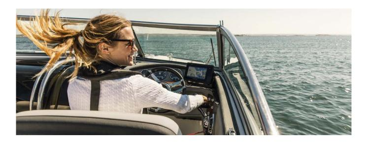
With the Trip computer, the driver gets access to information such as trip distance, average speed, fuel consumption and much more. The information easily monitored via the Volvo Penta displays.
